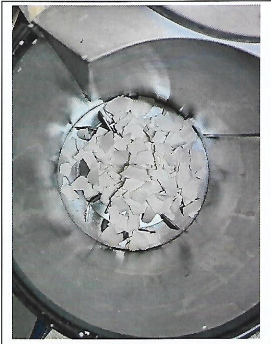
Slushing of Aqueous Coated Paper Board Sample in Hydrapulper
